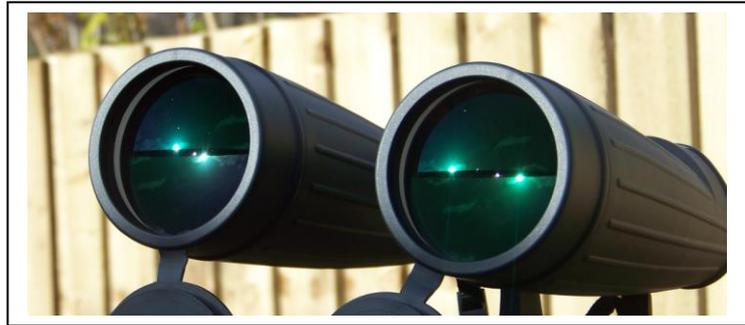
There are two minuscule cut-off segments in the light path, suggesting that the prisms are very slightly undersized, but not so much as to noticeably dim the image. They do not appear to be grooved on their hypotenuses.
