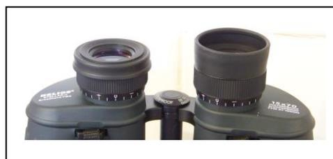
The lens coatings seem to be evenly applied and reduce the amount of reflected light. The manufacturer specifies that the optical transmission is 85%; this seems to be a realistic value. The insides of the objective tubes are ribbed along their entire length, suggesting that control of stray light should be good.
